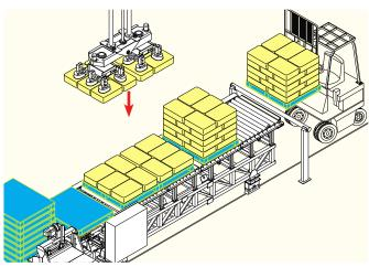
A forklift truck takes the full pallets from the roller way and deposits them in the pallet stock area.
