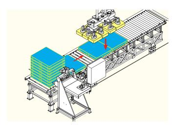
The empty pallets move onto the bag-loading roller ways.
