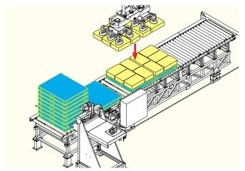
The automatic loader deposits the layers of bags on the pallets until the stack has been completed.
