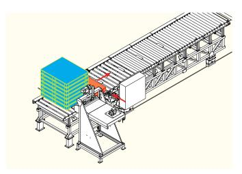
The pallet feeder lifts the stack of pallets and deposits the first empty pallet on the roller way. The pallet conveyed by the roller ways is positioned by the centering blades.
